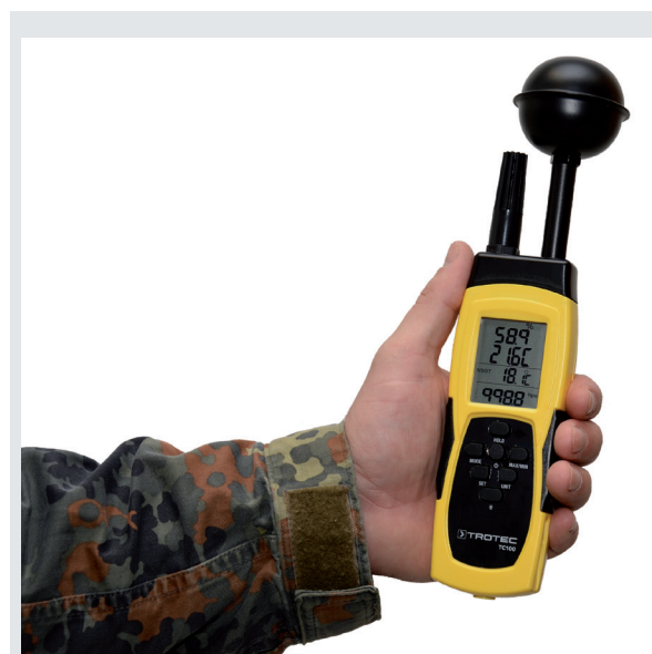
Fig. 2: Example of a commercially available climate measuring device that can be used to determine the Wet Bulb Globe Temperature (WBGT) as a climate index to assess the local current conditions.
